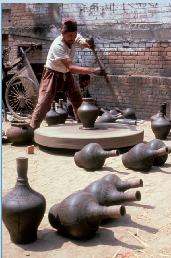
figure ar.2 The potter's wheel being used to produce a whole range of wares.
